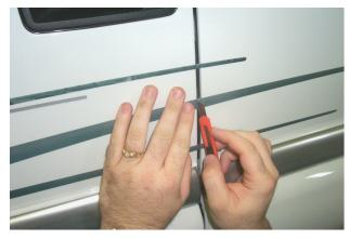
9. Trim away excess graphic material from door edges by inserting the knife along the edge of the opening at a 45-degree angle. Then carefully cut through the vinyl on both sides of the seam and remove the scrap.
