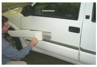
6. Remove the tape hinge from the center of the graphic. Remove the remaining backing paper, spray applications solution on the application surface and squeegee the remaining half of the panel onto the vehicle using the same method as outlined in Step 5.
