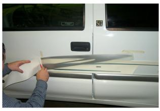
4. Temporarily secure the end of the graphic to the vehicle surface and cut the backing paper off near the center hinge.
