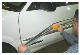
5. Lift the edge of the graphic from the vehicle surface and use the squeegee to rub the graphic into place using short, overlapping strokes from the center of the graphic to the end. By holding one end of the graphic off the vehicle surface as you squeegee, you will prevent air from becoming trapped underneath the graphic's surface.
