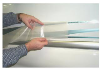
7. Remove the clear transfer masking by pulling it back at a 180-degree angle from the vehicle surface in a smooth steady motion.
